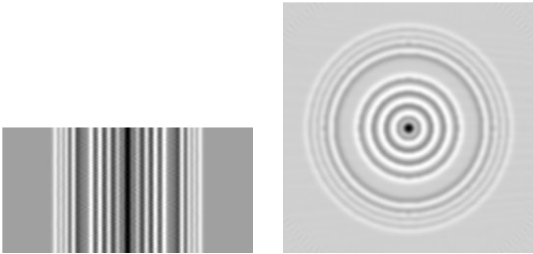
Figure 11: Sinogram and back-projected image for Laplacian of Gaussian with \sigma = 3.0
