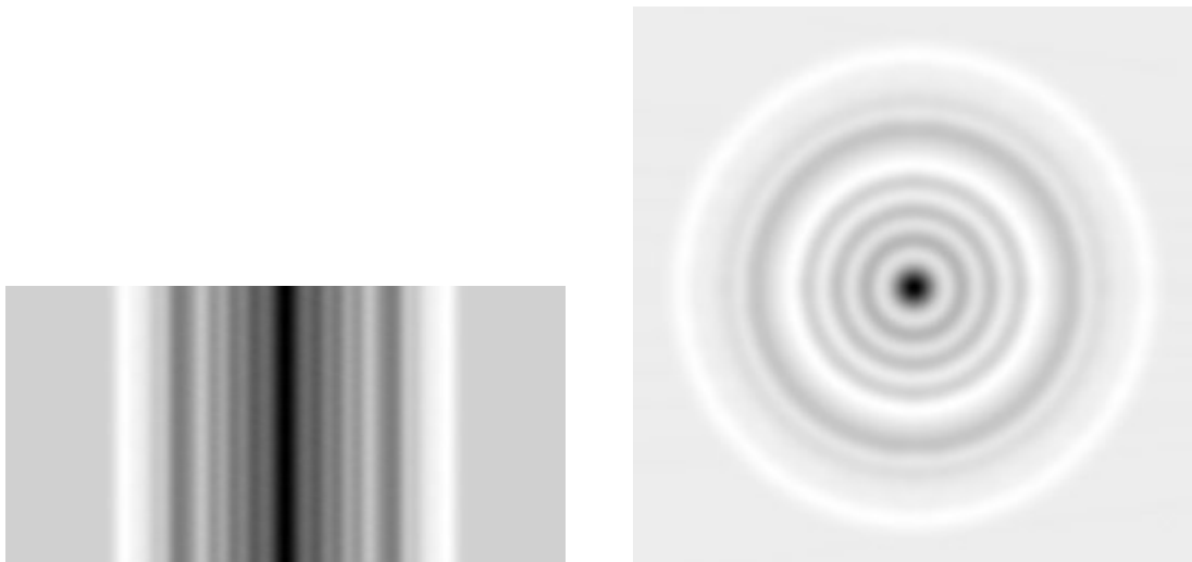
Figure 12: Sinogram and back-projected image for Laplacian of Gaussian with \sigma = 5.0
