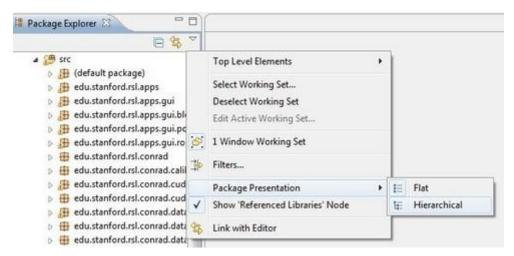
As CONRAD contains a lot of classes and packages, it is difficult to gain an overview for a beginner. Thus, we recommend to switch the package representation to "Hierarchical" as shown on the right. Click the small triangle on the top right of the package explorer to do so.
