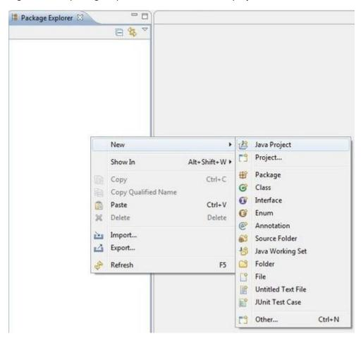
Once the normal layout of eclipse was loaded, the CONRAD project needs to be created. In a new workspace, the package explorer will show up empty. Right click the package explorer and create a new Java Project as shown on the right.
