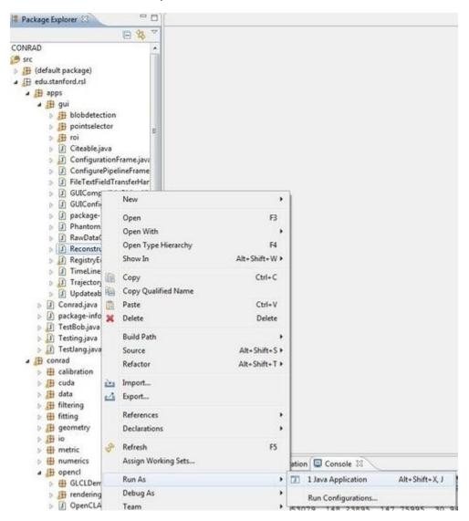
The main GUI of CONRAD is called Reconstruction Pipeline frame. It can be executed from the package explorer as shown on the right. Browse to the package "edu.stanford.rsl.apps.gui" and select the ReconstructionPipelineFrame. Right click it and select "Run As/Java Application".
