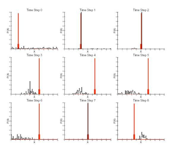
moving (sharp) Gaussian + uniform, N=100 particles
