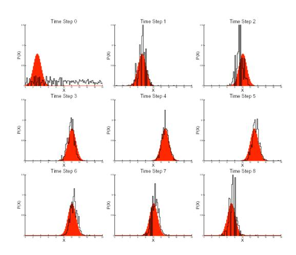
moving Gaussian + uniform, N=1000 particles
