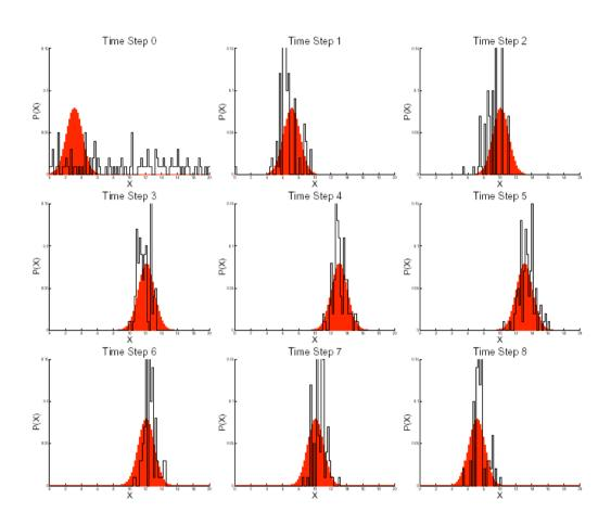
moving Gaussian + uniform, N=100 particles
