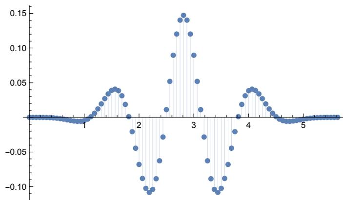
The scaling function belonging to the biorthogonal B spline filter partner for  $N=6$  and  $M=2$
