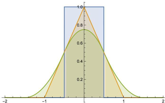
Computing the Fourier transform of the first N+1 B-spline functions
