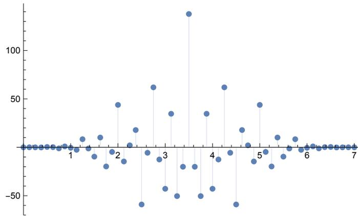
The wavelet function belonging to the biorthogonal B-spline partner filter for  $N=6$  and  $M=2$
