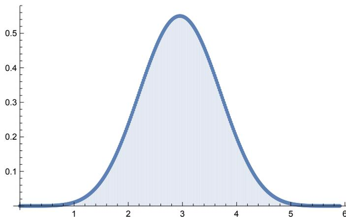
The wavelet function belonging to the B spline filter for  $N=6$
