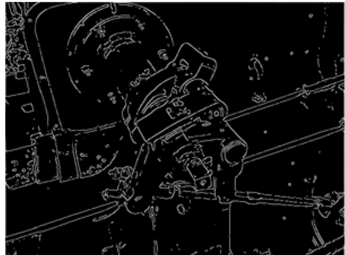
Step 4: Hysteresis thresholding final result
