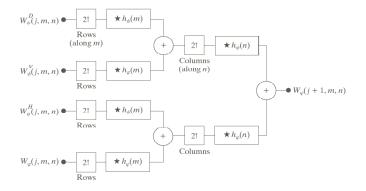
Figure: One level 2D HAAR WT as a filter bank (synthesis)
