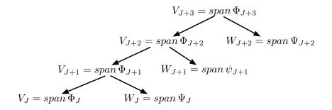
Figure: Scheme of a three-level Haar transform (analysis)
