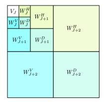
Figure: Coefficient scheme for a 2D-3-level-WT
