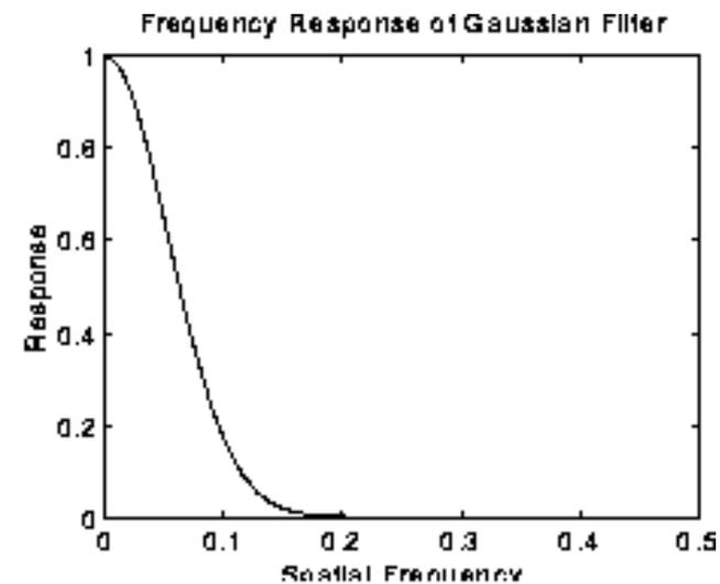
A close look at the frequency response of the two filters show that: compared to Gaussian filtering, mean filtering exhibits oscillations
