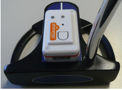
Figure 1. Placement and form factor of the SHIMMER sensor used in our system.
